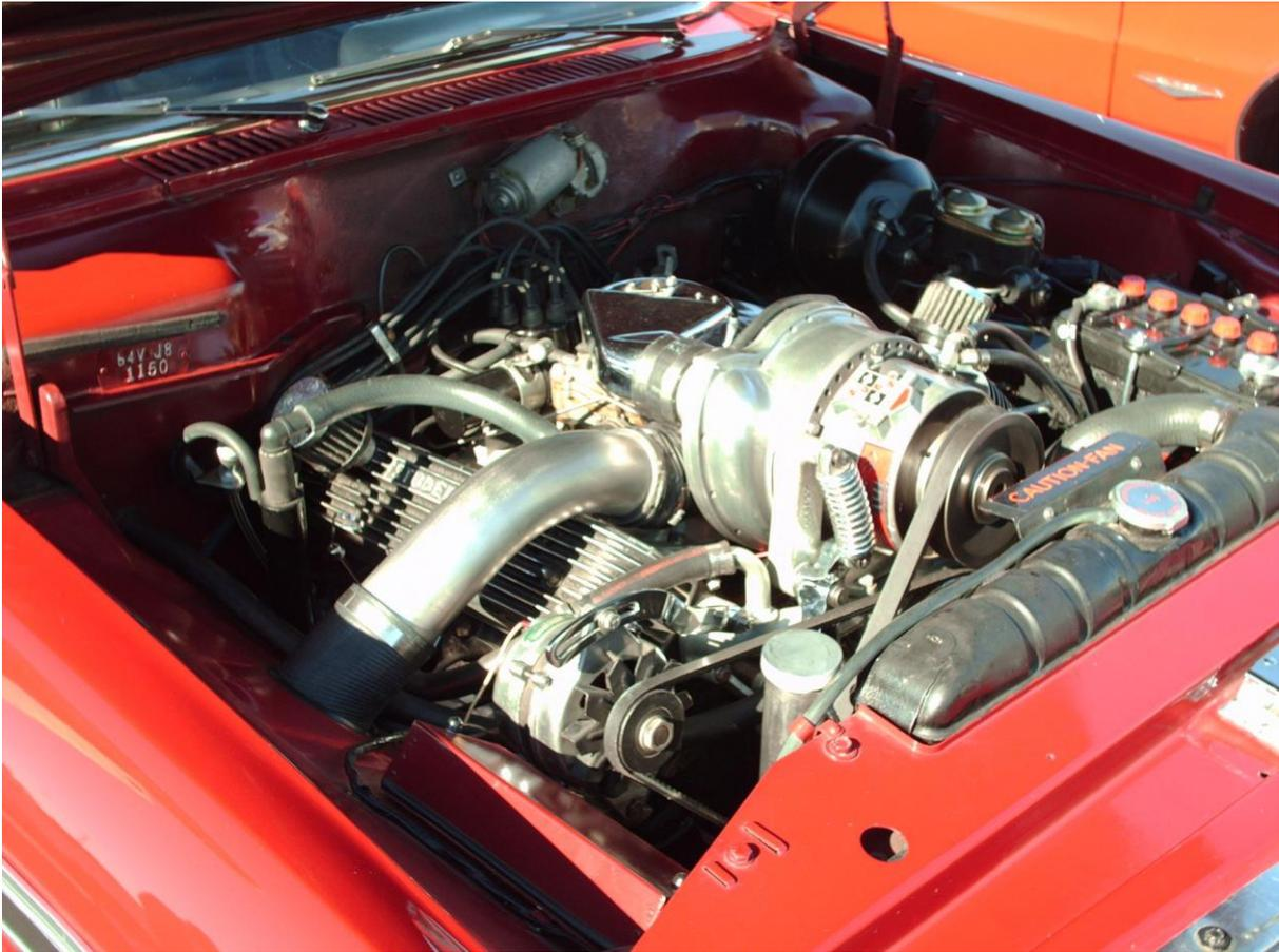
The R2 Avanti engine option included the Paxton Supercharger which was a very hot set-up for 1964. Dennis says that the configuration can still hold its own in the asphalt jungle.
